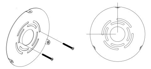
Mount the lamp base to the wall bracket using the three mounting screws
